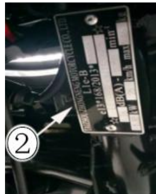
② The product nameplate is riveted on the right lower part of the frame.
